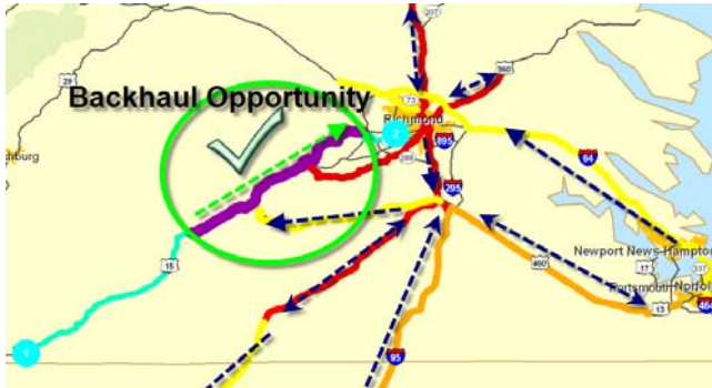
Figure 8. The green route indicates a tractor-trailer returning to a distribution center after delivering a primary shipment. The trailer is pulling no cargo, but can likely collaborate with a third party to pick up a full load in the purple region.
