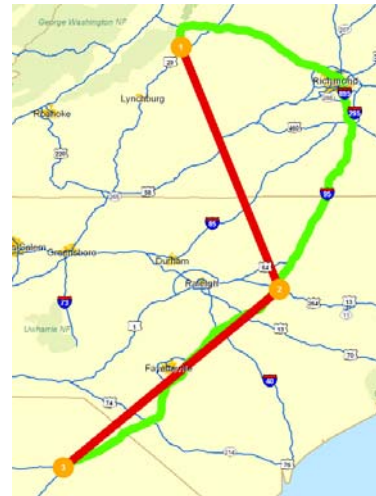
Figure 5. Orange circles depict a temporally ordered sequence of telematics messages. Red lines show straight-line distance, while the green line depicts an estimation of the route taken.
