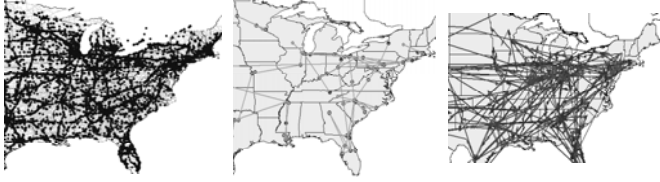
Figure 3. Visualization of (A) raw GPS data, (B) trips extracted -individual trailer, and (C) trips extracted -multiple trailers.
